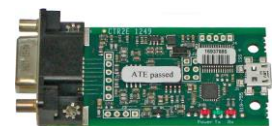
DSCUSBOEM1 The new PCB version with connectors and a 9 way D type slot and micro USB
