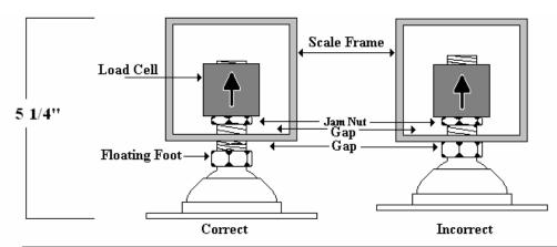
Please note the two examples above. These are end views of the load cells in your scale, (one at each corner). In the "Correct" example there is a gap between the floating foot (leveling leg) and the frame of the scale. In the "Incorrect" example there is no such gap and this condition WILL CAUSE THE SCALE TO WEIGH INACCURATE!
