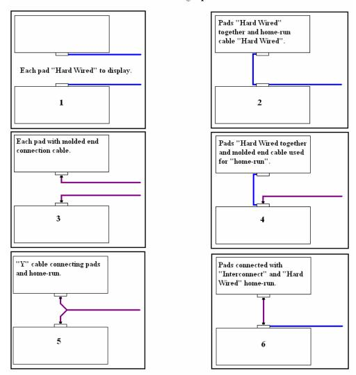
NOTE: All molded end cables are 4 pin with two exceptions. For use with either an LCIB or Portable Data Case 6 pin cables are required!
