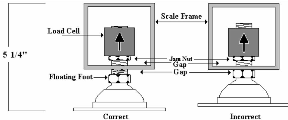
**Please note the two examples above. These are end views of the load cells in your scale, (one at each corner). In the "Correct" example there is a gap between the floating foot (leveling leg) and the frame of the scale. In the "Incorrect" example there is no such gap and this condition WILL CAUSE THE SCALE TO WEIGH INACCURATE!**
