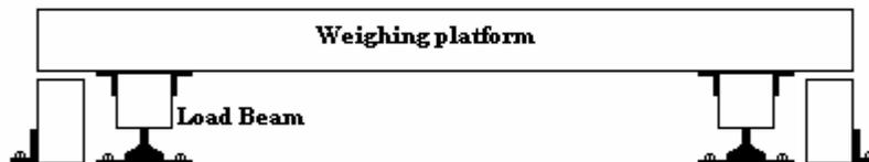
In this example the customer anchored a large wood block just under the end of the weighing platform at each end. He left about 1/4" gap between the top of the wood and the bottom of the weighing platform. With this setup it is important that the 1/4" gap is monitored on a regular basis as the feet can turn up into the load cell under high vibration applications. Please note that only up and down movement is checked with this setup.
